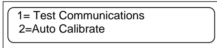
While in the second SETUP screen, pressing "1" will test the communications with another controller if they are interfaced together. If there is no communications, the messages "No Data Received" and "No Data Sent" will be seen.
