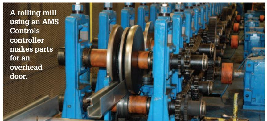
**A rolling mill using an AMS Controls controller makes parts for an overhead door.**
